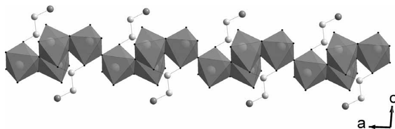
Figure 2. A polyhedral and ball-and-stick representation of the \{\text{Mo}_4\text{O}_{13}(\text{NH}_3\text{CH}_2\text{COO})_2\}_n chain in compound 1 ; medium gray polyhedra belong to \text{MoO}_6 octahedra, ball-and-stick belong to Gly ligands, hydrogen atoms are omitted for clarity.
